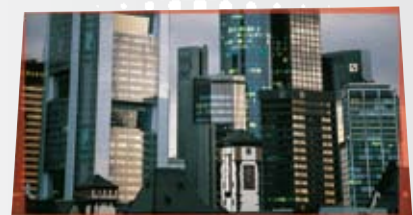
Trapezoidal distortion (projector a little to the left and too high); red margin is off the screen.
